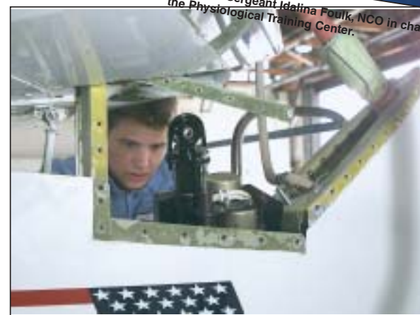
Photo by Budd Butcher Clint Calnan, 84th Air Lift Flight, replaces a horizontal stabilizer actuator on a C-21 aircraft.
