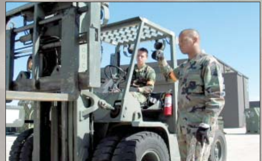
Airman Miralem Bekric (left), a 21st Logistics Readiness Squadron cargo passenger service worker, follows Master Sgt. Ronald Lacy's, NCO in charge of the cargo deployment facility, spotting signals to properly adjust the forklift tines for cargo processing.
