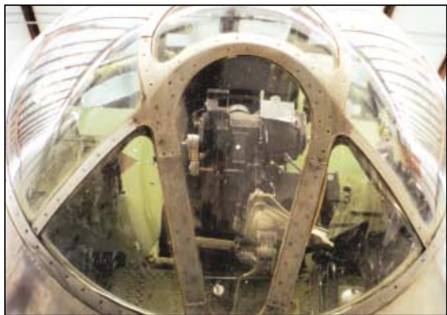
The B-29 aircraft is equipped with a Norden bombsight.
