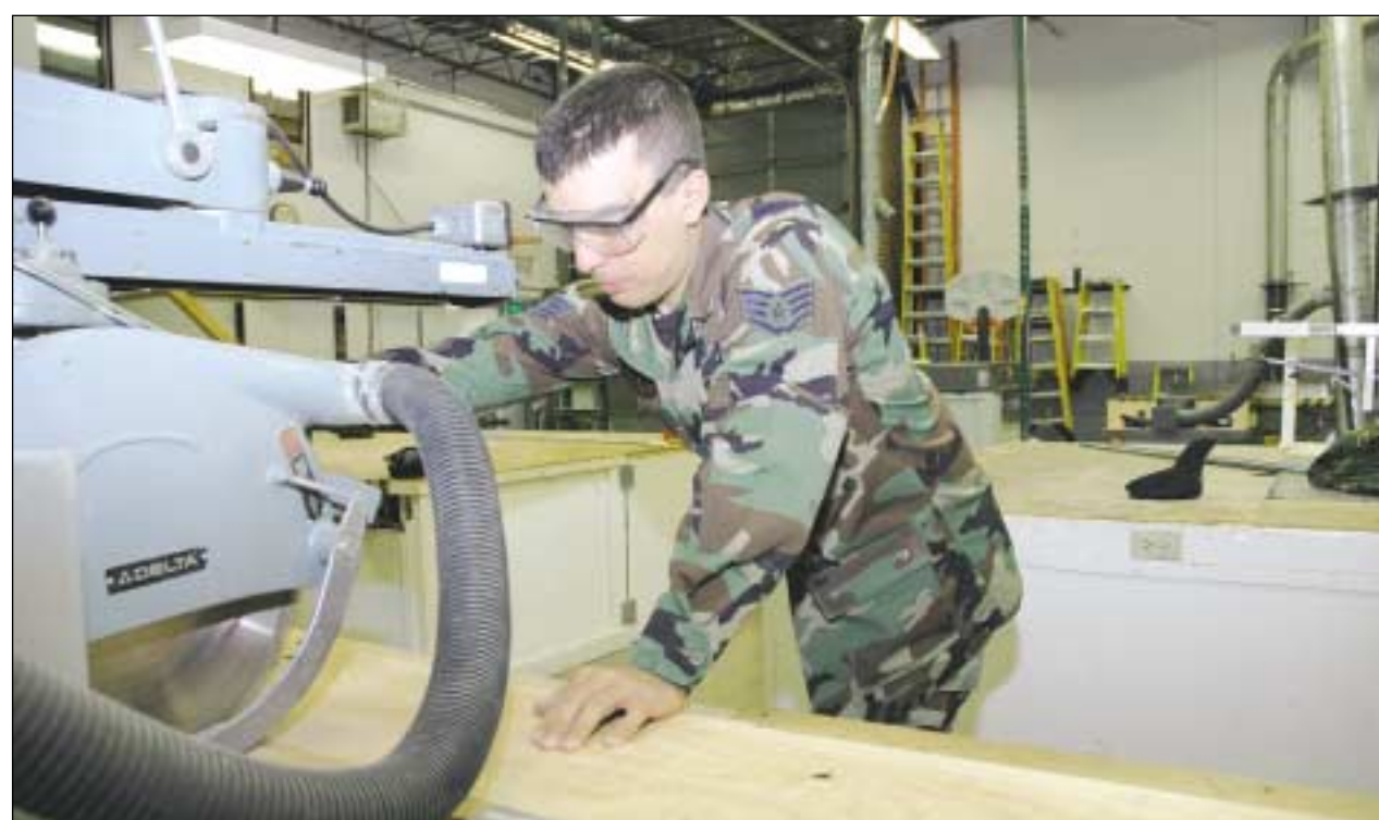
Staff Sgt. David Wilson, structural journeyman, lines up the blade on the radial arm saw before making the cut.
