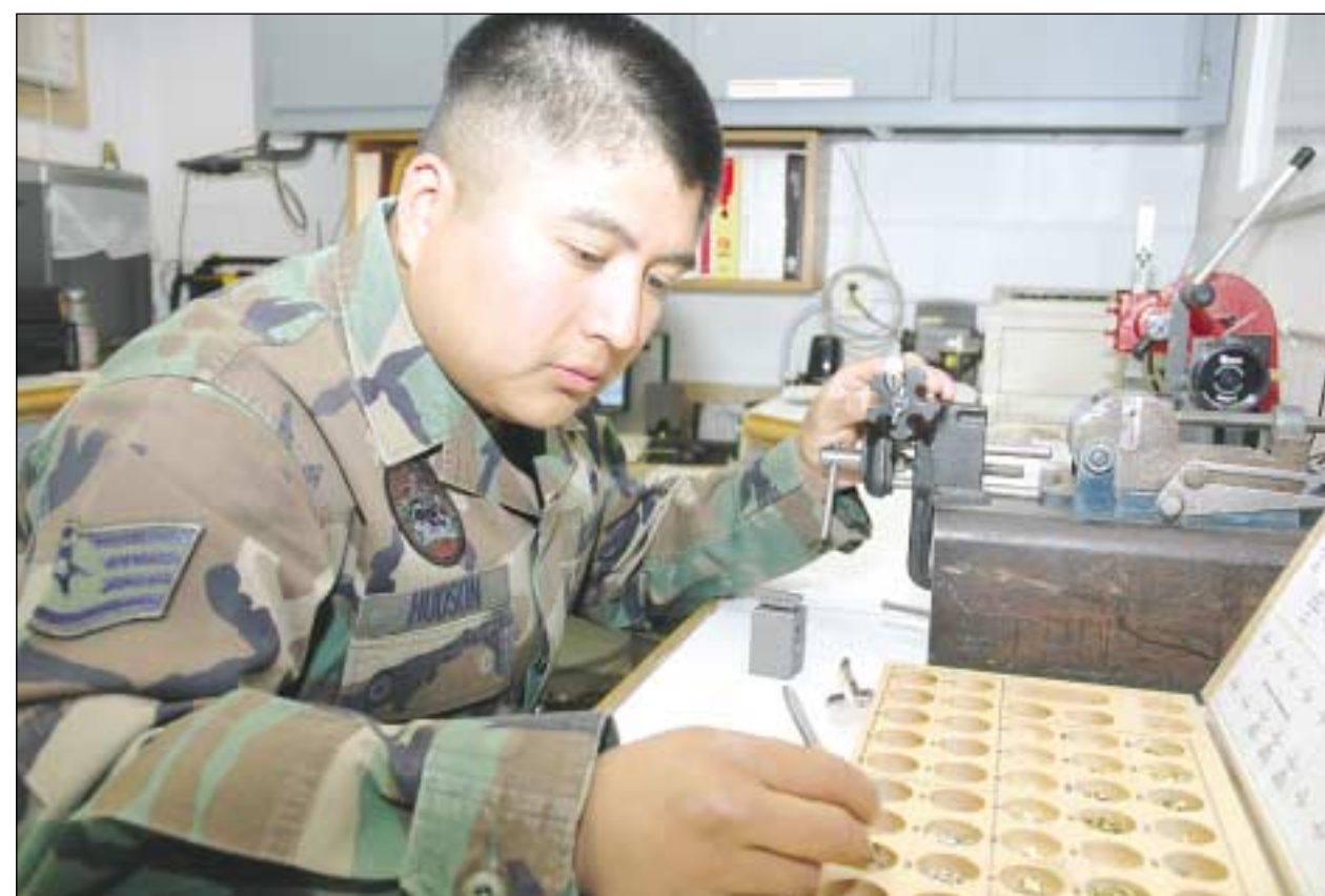
Staff Sgt. Selvin Hudson, structural journeyman, selects the proper pin size before cutting a new key.
