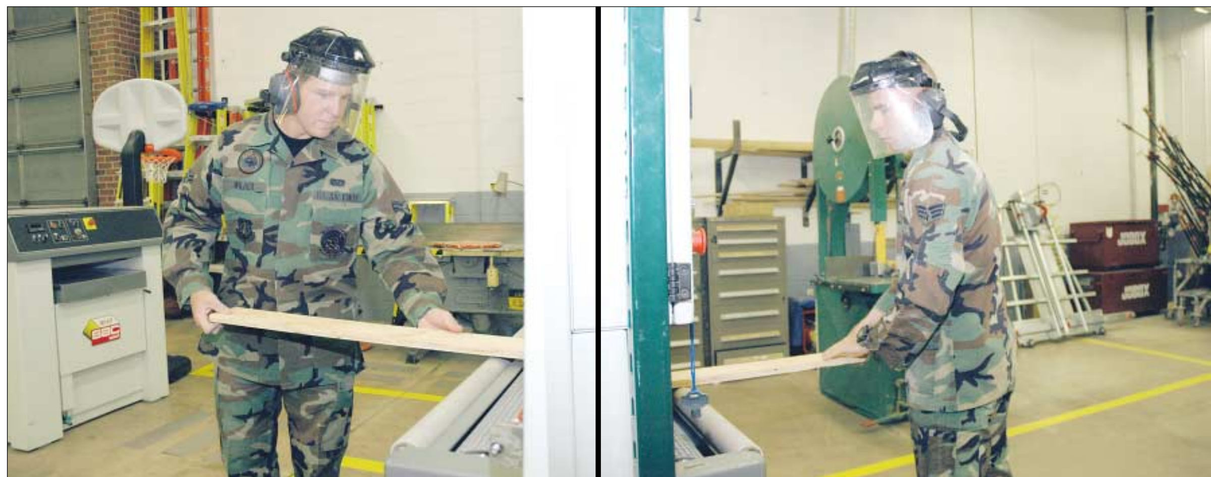
Airman 1st Class Louis Wilder, structural apprentice, receives a board fed through the surfacer from Senior Airman Charles Kropog, structural apprentice. Teamwork is a key to getting the job done right.
