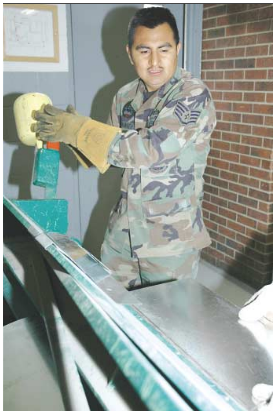
Staff Sgt. Jose Hernandez, structural journeyman, checks the alignment before making a critical sheet-metal bend.
