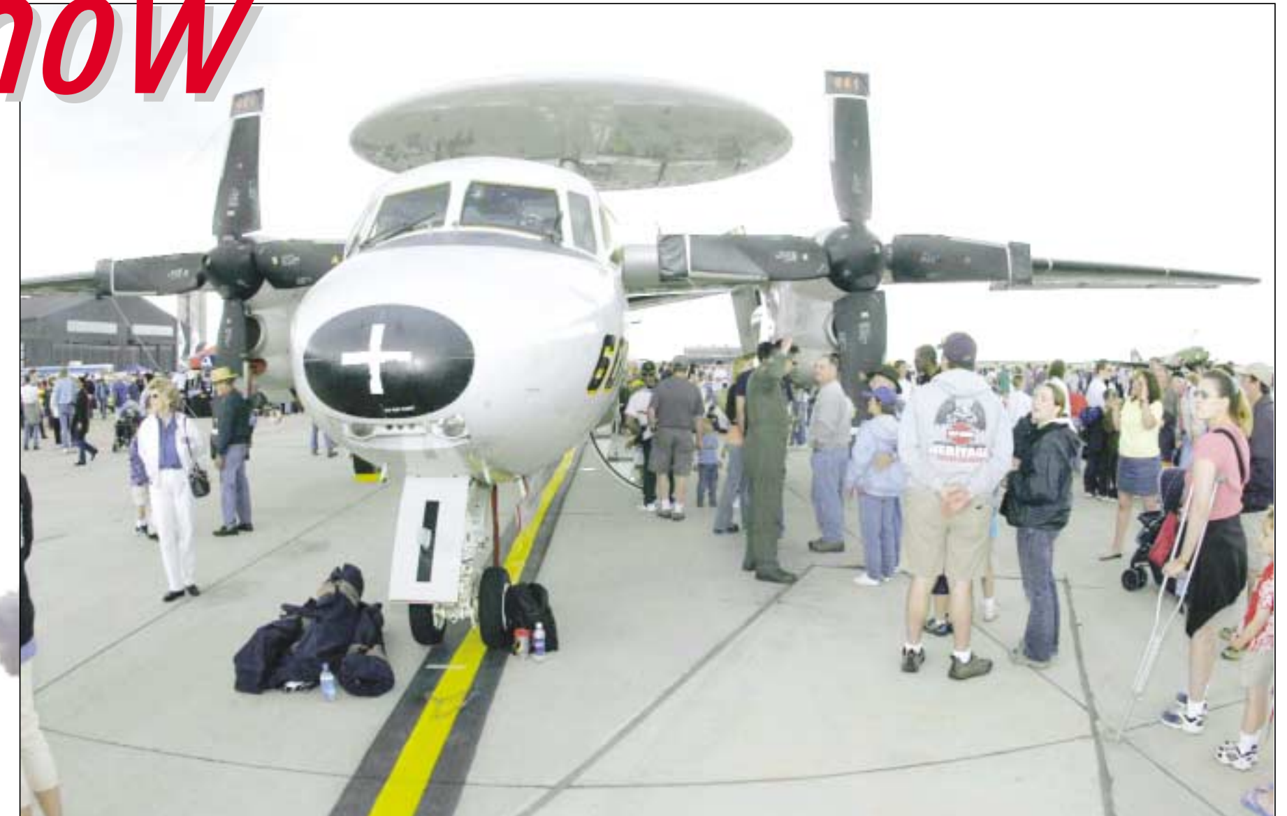
Air show attendees investigate a Navy E-2 Hawkeye. The Hawkeye is the Navy's all-weather, carrier-based tactical battle management airborne early warning command and control aircraft.
